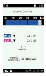
Verify the "Acoustic Calibration" is displayed in the upper part of the screen.
