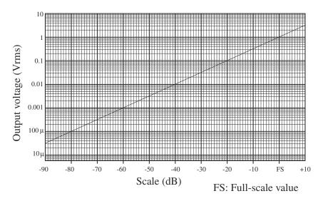
Ideal characteristics of the display value and the output voltage
